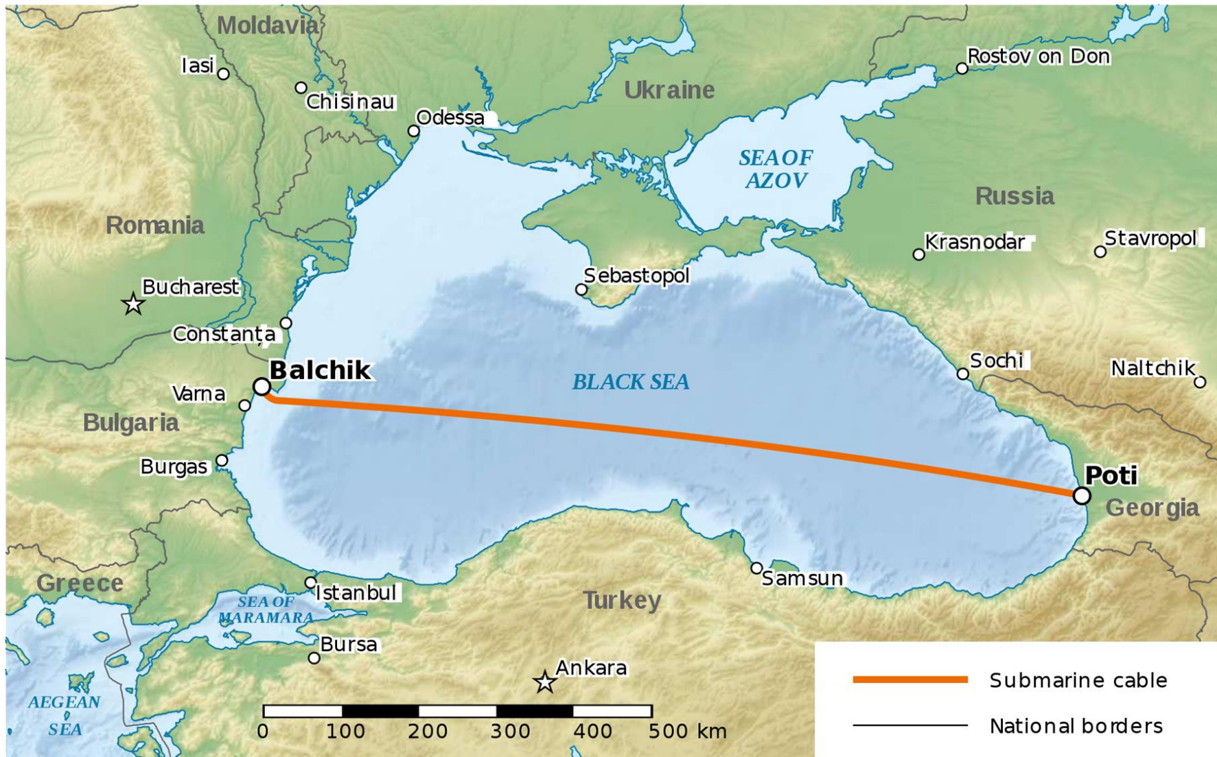
CAUCASUS CABLE SYSTEM GEORGIA-BULGARIA The only communication cable linking Georgia to Europe
